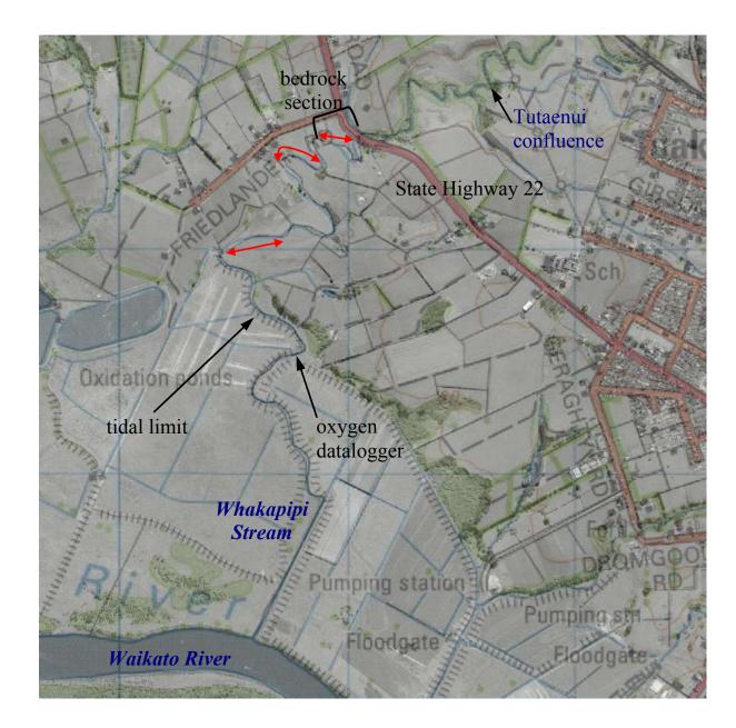
**Figure 2.1:** The lower Whakapipi Stream, between the Tutaenui confluence and the Waikato River. Habitat was surveyed at 15 cross-sections, with three groups of 5 cross-sections indicated by red arrows on the map. Oxygen was monitored at the site indicated and the tidal limit was also assessed. Flood control stop-banks are indicated by hatching. Note that the oxidation ponds do not discharge to the Whakapipi Stream. The aerial photo and topomap overlay were sourced from Maptoaster software.
