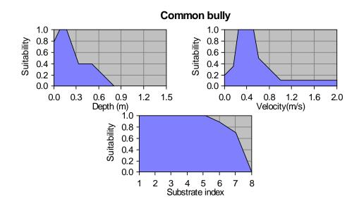
**Figure 1.7:** Habitat suitability curves for common bully, where suitability ranges from 0 (unsuitable) to 1 (optimal). Substrate index: 1=vegetation, 2=silt, 3=sand, 4=fine gravel, 5=gravel, 6=cobble, 7=boulder, 8=bedrock (Jowett & Richardson 1995).
