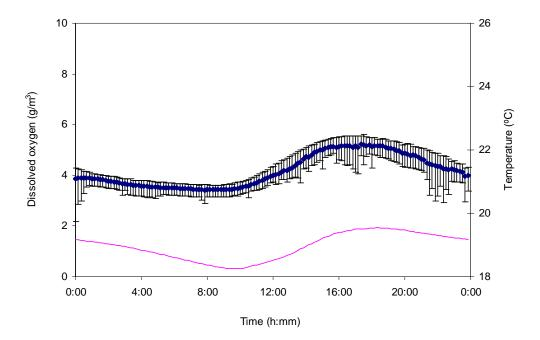
**Figure 3.6:** Dissolved oxygen concentrations in the Tutaenui Stream at Hamilton Bridge. Oxygen concentrations were averaged for each time of day over the monitoring period (2 to 12 March 2007) to give the average 24-hour cycle of dissolved oxygen. Bars show the maximum and minimum for each time of day. The average temperature for each time of day is also presented (lower line).
