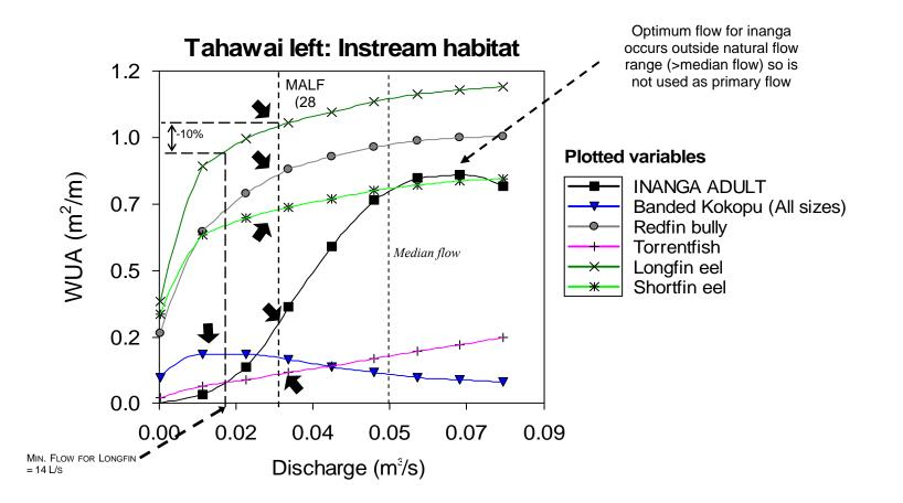
**Figure 1:** Modelled habitat for the Tahawai Stream (western BOP) expressed as habitat (WUA m<sup>2</sup>/m) versus flow. Primary flows determined using established criteria are arrowed for each species. Minimum flow calculation for longfin eel illustrated. Note, this is presented as an example only, as taxa and baseflow estimates were altered to illustrate the method.
