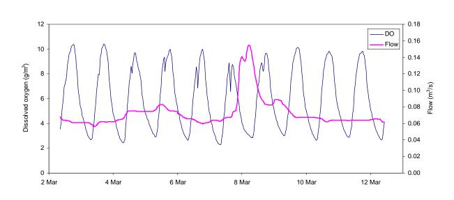
**Figure 3.2:** Dissolved oxygen and flow results for the Whakapipi Stream (March 2007). Dissolved oxygen was monitored in the tidal lowland reach and flow monitored by Environment Waikato at State Highway 22 (2 km upstream).
