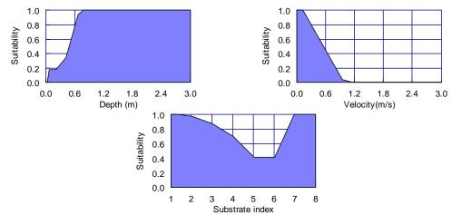
Longfin eels <300 mm (Jellyman et al. 2003) 1.0 1.0 0.8 0.8 Suitability Suitability 0.6 0.6 0.4 0.4 0.2 0.2 0.0 0.0 3.0 0.0 0.6 1.2 1.8 2.4 3.0 0.0 0.6 1.2 1.8 2.4 Depth (m) Velocity(m/s) 1.0 0.8 Suitability 0.6 0.4 0.2 0.0 3 4 5 6 Substrate index 2 6 7 8 1
