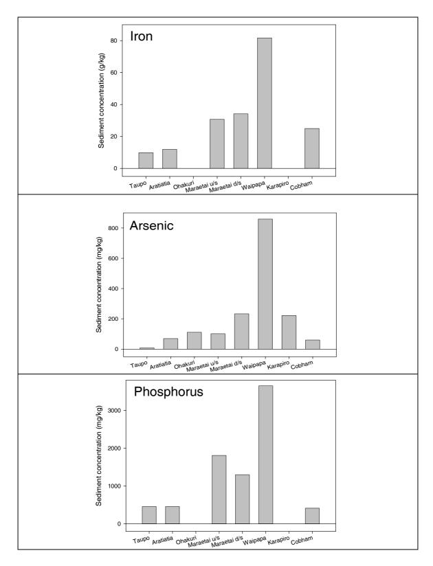
Figure 3 Concentrations of iron, arsenic and phosphorus reported for sediment samples collected from Waikato River lakes in the AEE [4, p 101]. Arsenate  $(AsO_4^{3-})$  and phosphate  $(PO_4^{3-})$  share a similar adsorption chemistry and are strongly adsorbed by iron (and manganese) oxides.
