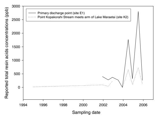
Figure 2 Reported concentrations of total resin acids (µg/L) in wastewater at sampling site E1 and Kopakorahi stream water at sampling site K2.
