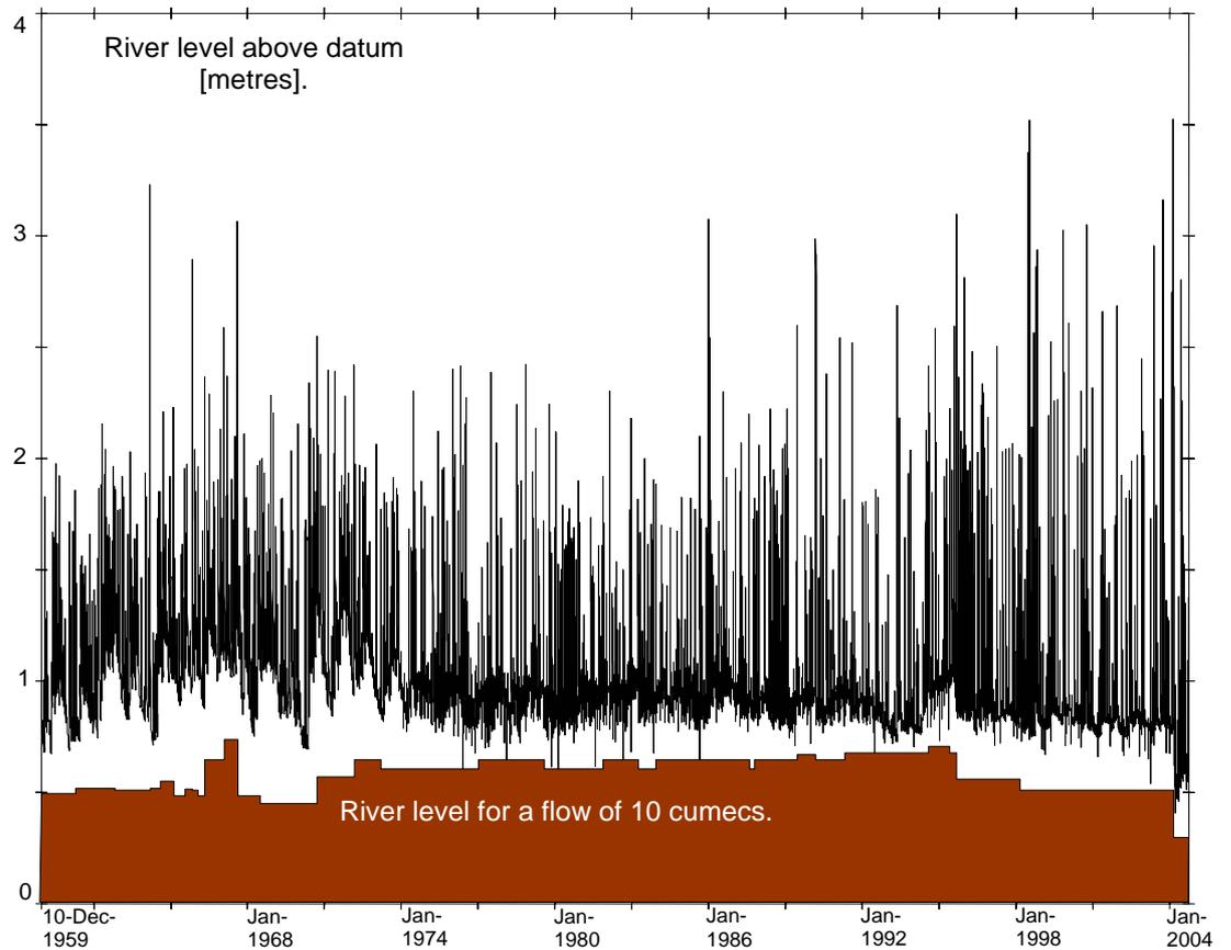
**Figure 5: Changes in water level at Puketarata gauging station.**
