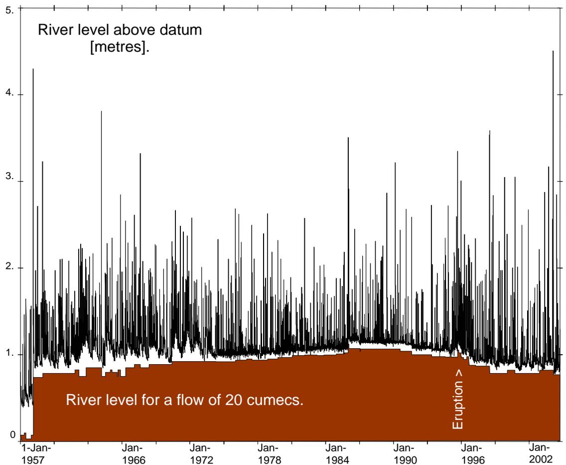
**Figure 6: Changes in water level at Turangi gauging station.**
