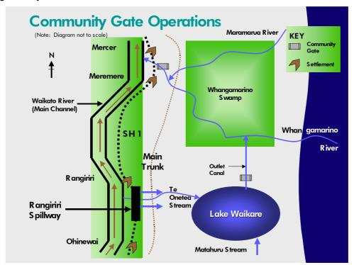
Figure 1: The location and operating design of the Lower Waikato Community Gates.
