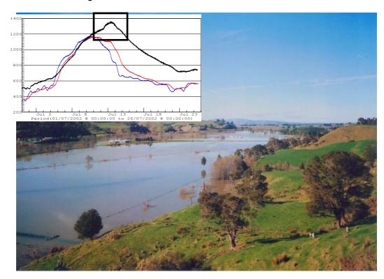
Figure 3: Flooded farmland at Mercer. Inset: Waikato River levels recorded at Ngaruawahia, Rangiriri and Mercer (bottom to top respectively). The 'box' indicates the effect of a last minute rainstorm which coincided with the primary peak.
