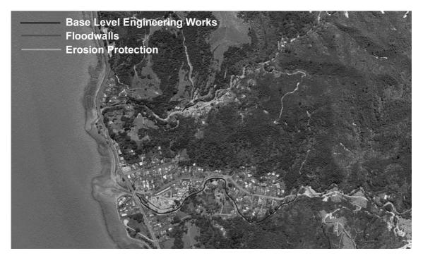
Figure: Full engineering works on the Waiomu Stream and Pohue Stream
