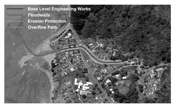
Figure: Intermediate engineering works on the Tararu Stream
