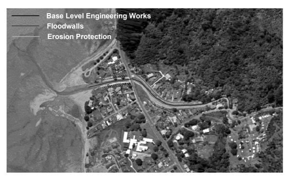
Figure: Full engineering works on the Tararu Stream
