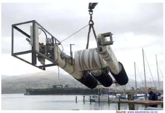
The experimental wave energy converter, which has been trialled in Lyttelton Harbour by Wave Energy Technology, seeks to harness both kinetic and potential energy from passing waves.
