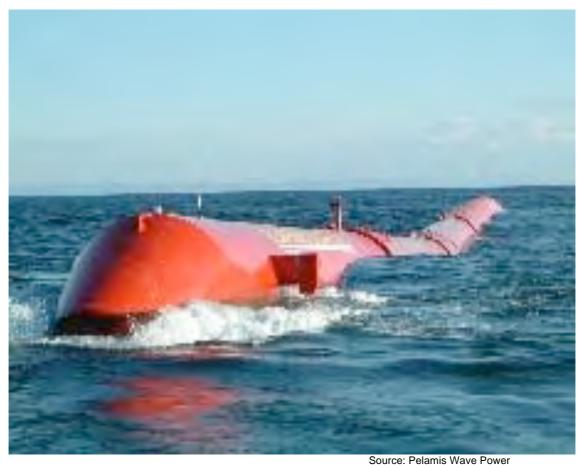
The Pelamis system, when arrayed in a cluster of units, can produce 30 MW over a square kilometre of ocean, and has the potential to power 20,000 homes. It is already on trial in Portugal and the United Kingdom. There are proposals to import and manufacture this technology in New Zealand, which could be deployed off the Waikato's west coast.
