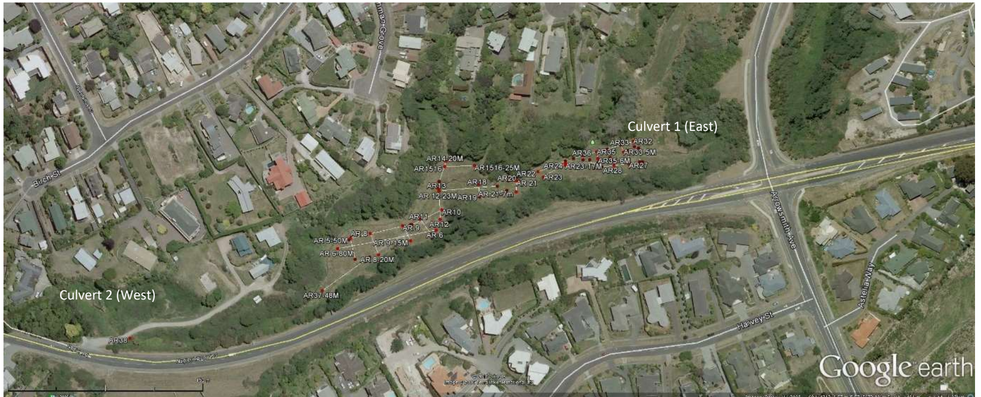
Figure 2: Overview of all GPR transect lines and their distribution at Armstrong Reserve.
