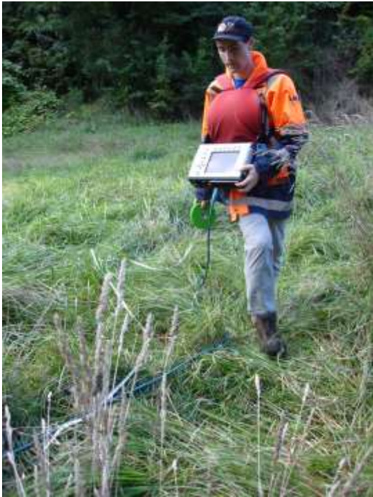
Figure 2: A SIR 3000 control module was used to collect GPR data.
