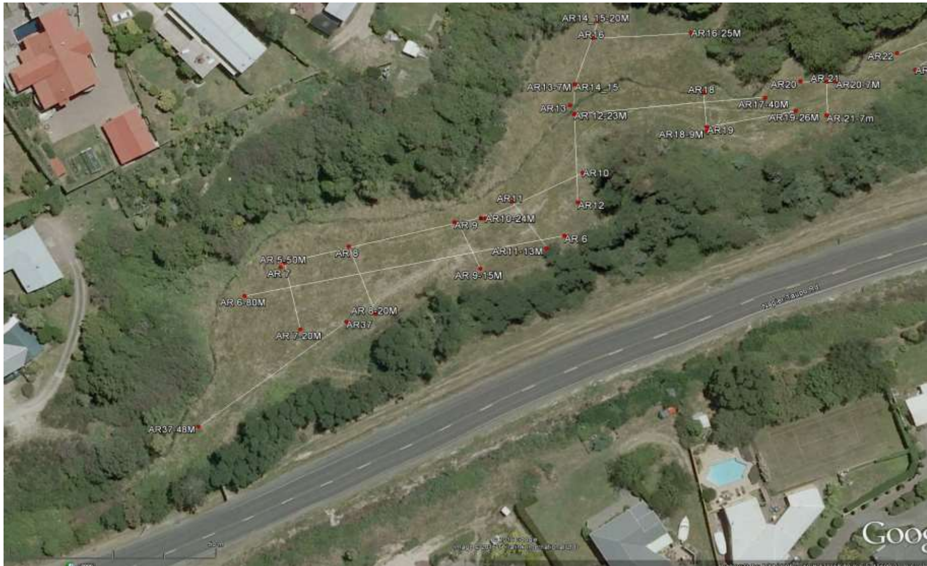
Figure 3: Overview of the western section of the study area showing individual GPR transect lines.
