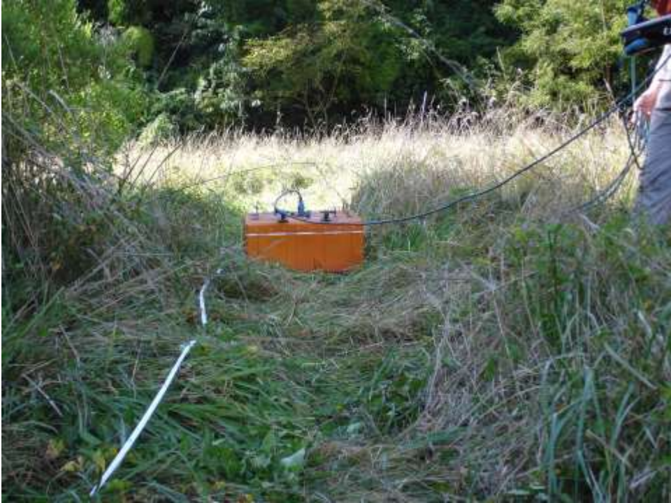
Figure 1: The Ground Penetrating Radar (GPR) unit imaged the subsurface using a 200 MHz GSSI antenna.
