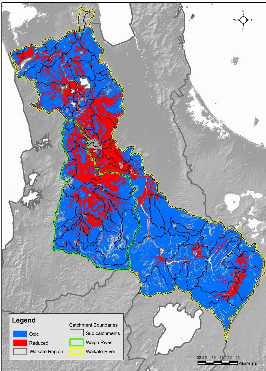
Figure 2: Map of predicted redox status for medium depth (25 - 100 m bgl) groundwater overlaid on sub-catchment boundaries for Waikato catchment.
