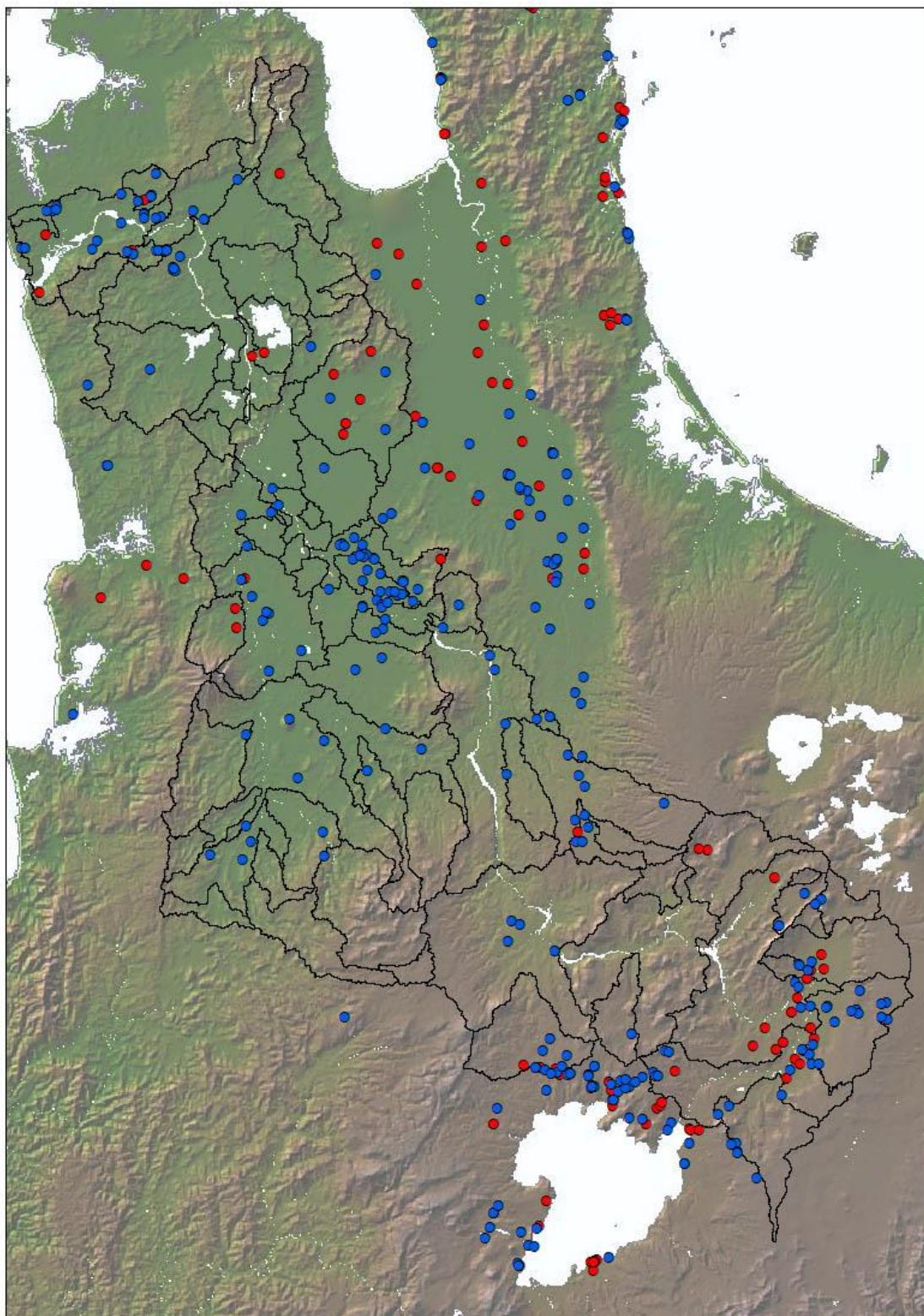
Figure 3: Location of wells used for developing models for prediction of groundwater redox status overlaid on sub-catchment boundaries for Waikato catchment. Blue circles are wells with oxidised groundwater; red circles are wells with reduced groundwater
