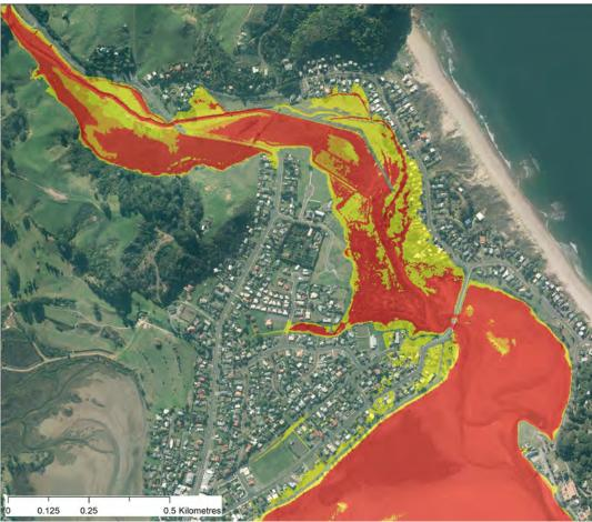
Figure 18 Post-Scheme 1%AEP (100 year ARI) river flood hazard classification map for Grahams Creek with a projected 0.5 m sea level rise
