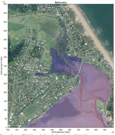
Figure 9 Tidal inundation during design high tide
