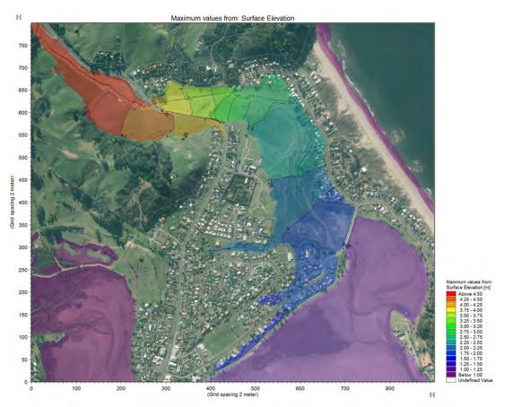
Figure 6 Predicted inundation for the pre scheme 100y flood levels (relative to Moturiki vertical Datum)
