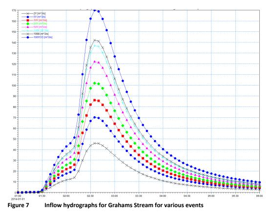
Figure 7 shows the inflow hydrographs for the various events applied to the hydraulic model.
