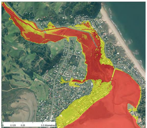
Figure 21 Post-Scheme 1%AEP (100 year ARI) river flood hazard classification map for Grahams Creek with a projected 1.2 m sea level rise
