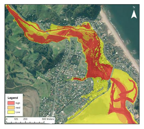
Figure 16 Pre-Scheme current climate 1%AEP (100 year ARI) river flood hazard classification map for Grahams Creek.
