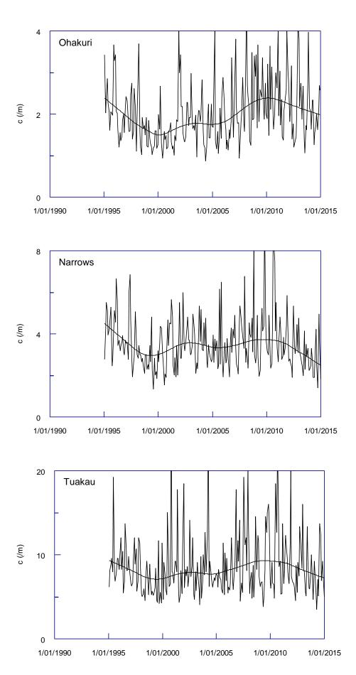
**Figure 7**: Monthly estimates of beam attenuation (*c*) in the Waikato River at Ohakuri, Narrows and Tuakau, 1995–2014. LOWESS smoothing curves have been fitted to the data.
