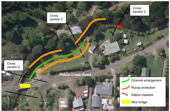
Figure 9 Completed engineering works at Pohue Stream
