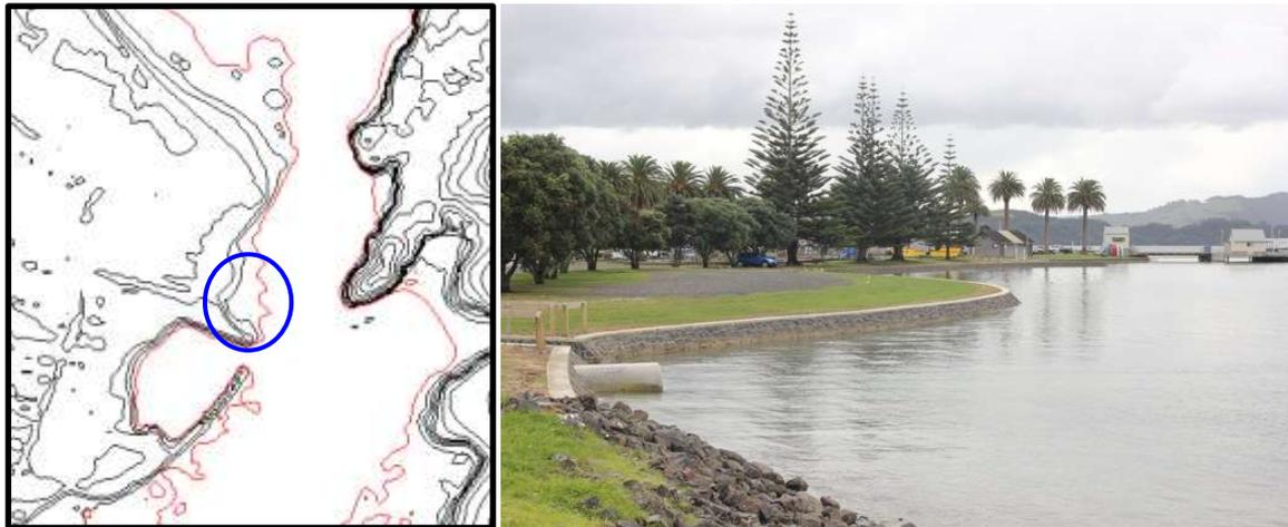
**Figure 3.22** The model bathymetry along the Whitianga water front (left) and a photo of the area (right). The photo was taken from a location approximated by the blue oval. The red is the 0 m contour, black contours are in 1 m intervals. Photo was taken between 1 and 2 pm on May 16, 2012 when the tide stage would have been at approximately +1.5 m relative to MLLW (<http://www.tides4fishing.com/nz/coromandel/whitianga>).
