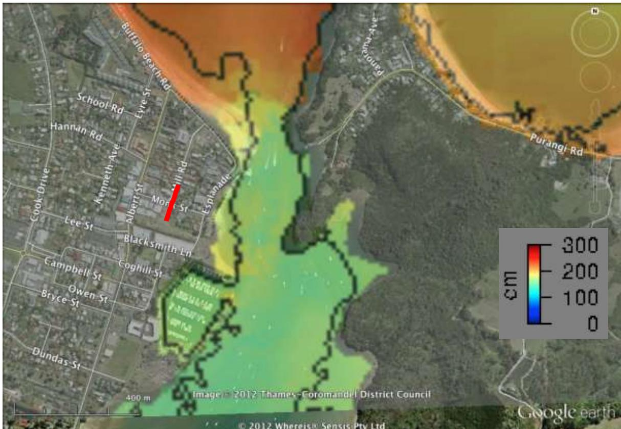
**Figure 3.21 Modelled inundation overlaid on an aerial image of the Whitianga waterfront. The red line indicates the approximate observed extent of inundation in 1960.**
