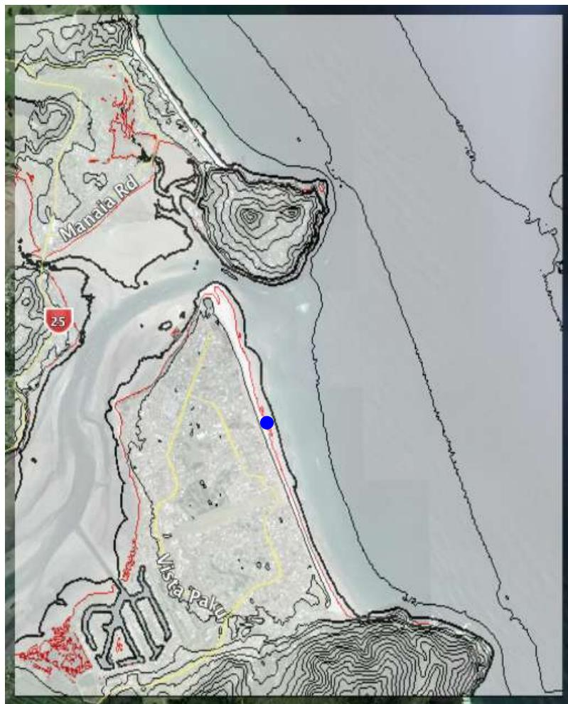
**Figure 4.1** The Tairua topography DEM over aerial imagery. The photo shown in below was taken from the location indicated by the blue dot with a view to the southeast. The thicker black line is the 0 m contour while the red line is the +1 m elevation. Thinner black contours are at 5 m intervals.
