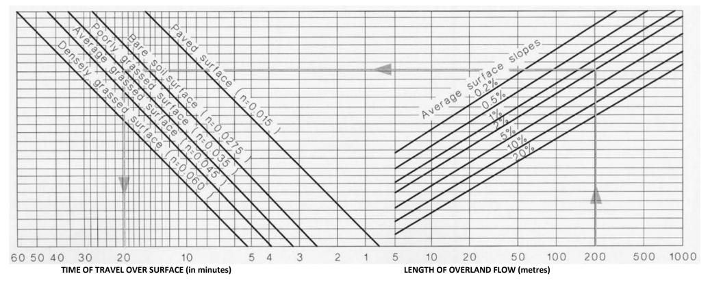
Example: For surface water flowing 200 m over an average grassed surface at a slope of 2% the time of travel is 20 minutes
