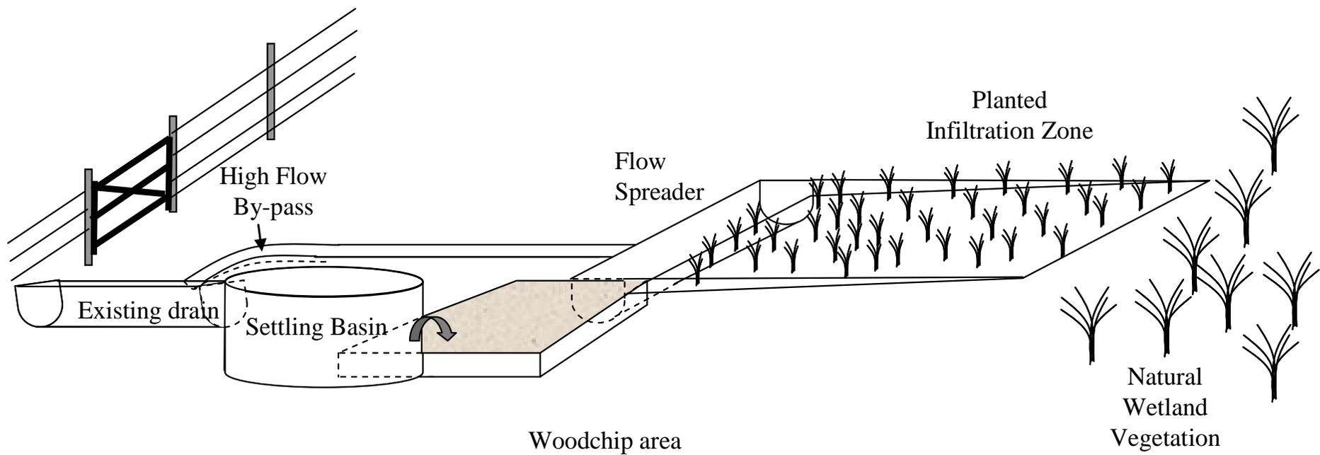
**Figure 27:** Infiltration system based on Lake Serpentine (Sukias et al., 2006) modified to include a woodchip area.
