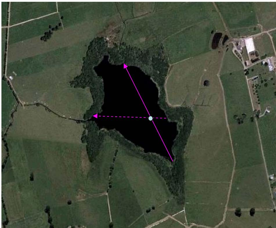
**Figure 4:** Lake Mangahia sonar transects with the solid line being Transect A and the dotted line being Transect B. The dot was the area of the deepest readings.
