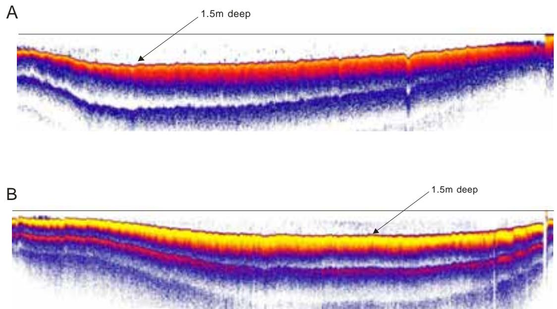
**Figure 5:** Lake Mangahia sonar transects: A running south – north and B running east – west (see Fig. 4 for locations) showing a shallow lake with a maximum depth of 1.5 m and a profile with low slope.
