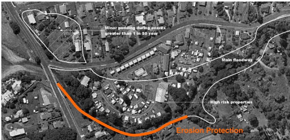
Figure 14 Proposed erosion protection
