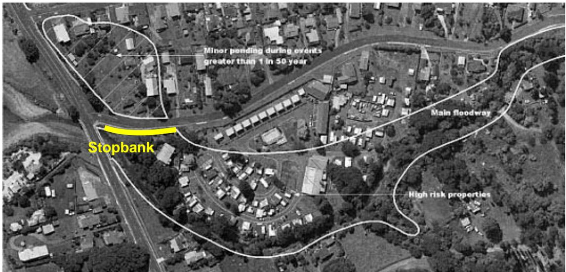
**Figure 6 Proposed downstream stopbank**
