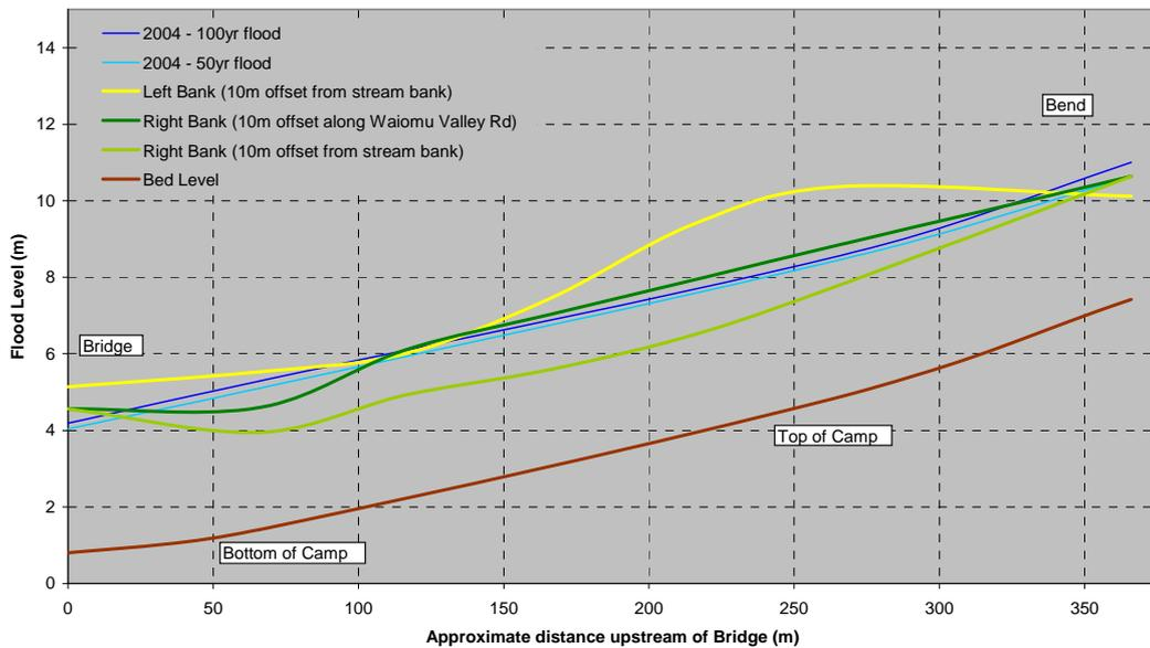
**Figure 11 Ground levels and existing flood levels adjacent to campground**
