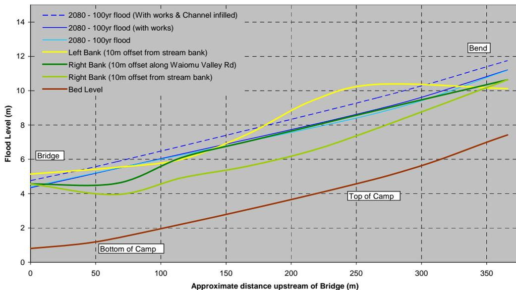
**Figure 12 Ground levels and future flood levels adjacent to campground**
