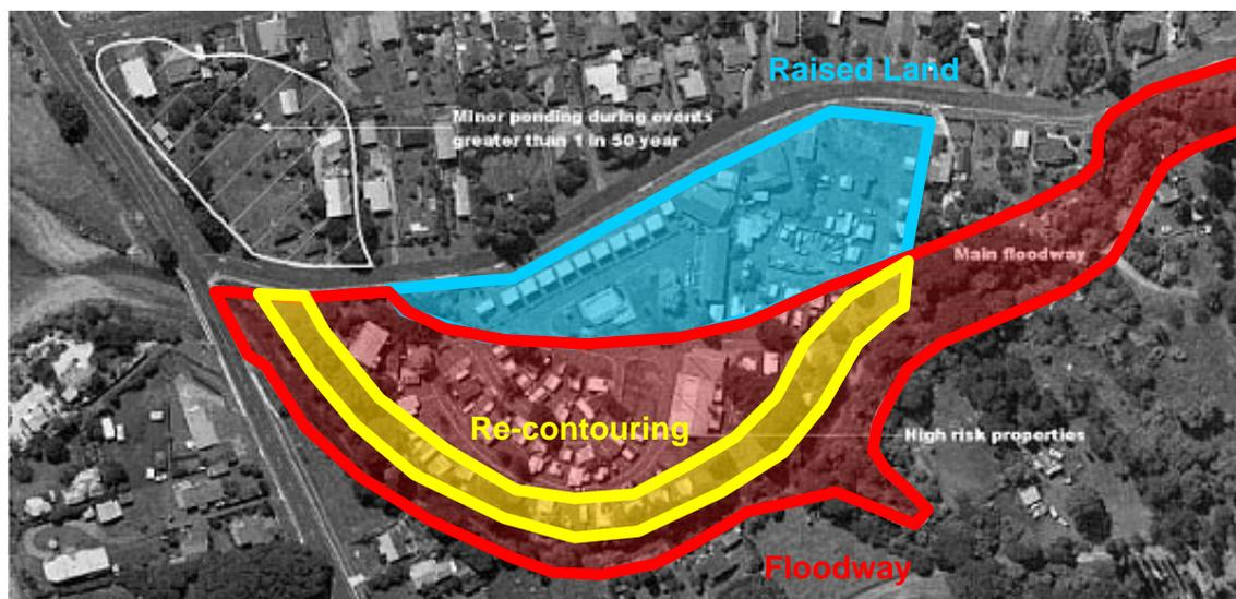
**Figure 10 Proposed floodway works**
