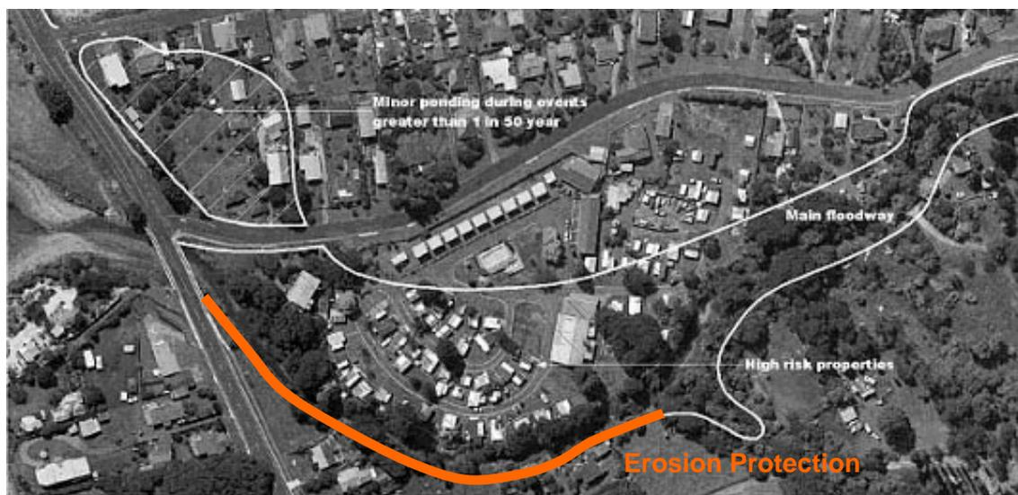
**Figure 4 Proposed erosion protection**
