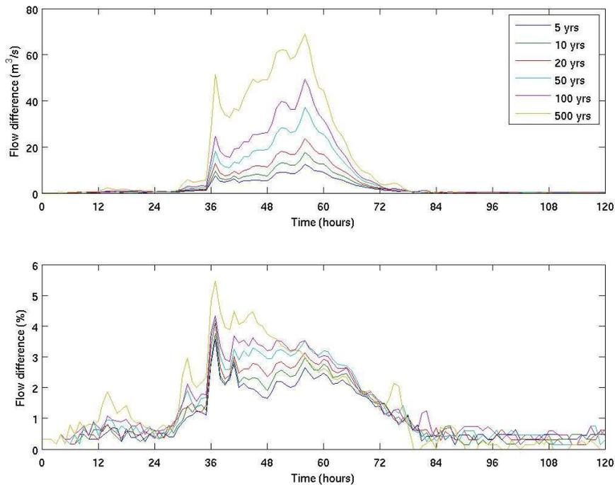
**Figure 31:** Difference in simulated Taupo-Karapiro inflow due to land use change for the 6 storm scenarios. Differences are expressed as changes in  $m^3/s$  (top graph) and percent (bottom graph) relative to the current land use scenario.
