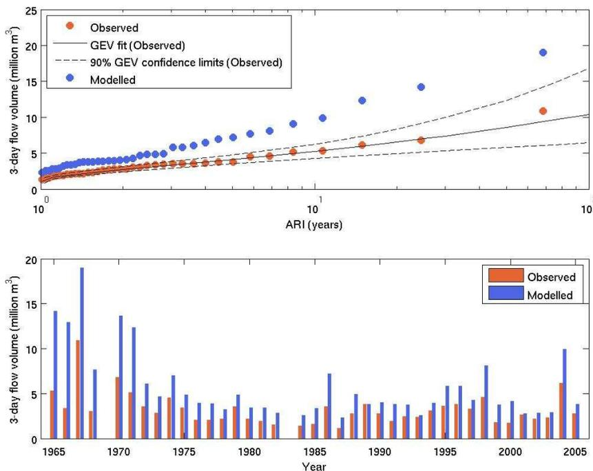
**Figure 12:** Modelled and observed annual maximum 3-day floods for Waiotapu at Reporoa. Upper panel: Annual series; lower panel: Flood frequency analysis - analysis of observations by SKM (Thornburrow & Mulholland 2009).
