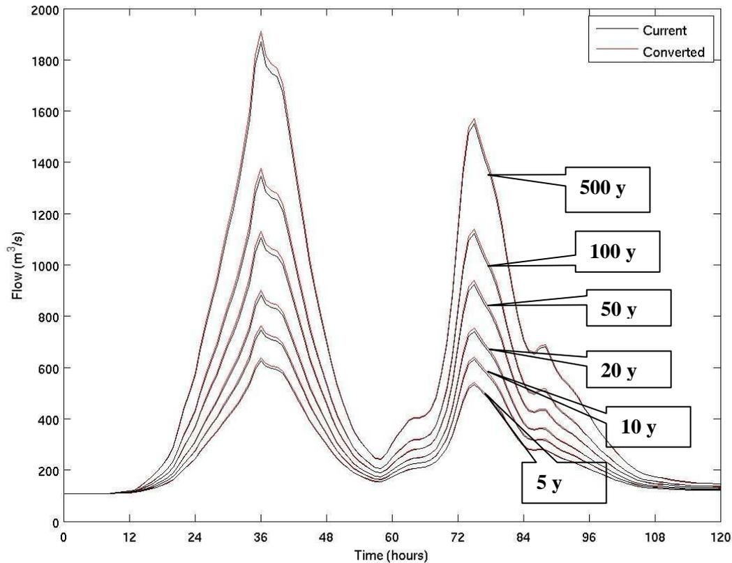
**Figure 25: Simulated Taupo-Karapiro inflow hydrographs for the 6 synthetic rainfall events under current (black) and converted (red) land use scenarios.**
