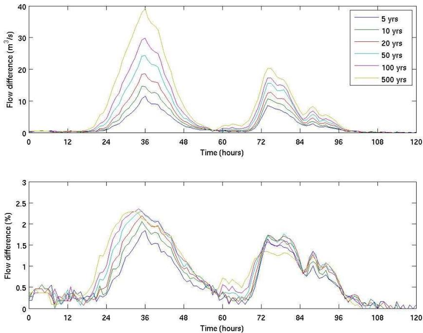
**Figure 26:** Difference in simulated Taupo-Karapiro inflow due to land use change for the 6 storm scenarios. Differences are expressed as changes in  $m^3/s$  (top graph) and percent (bottom graph) relative to the current land use scenario.
