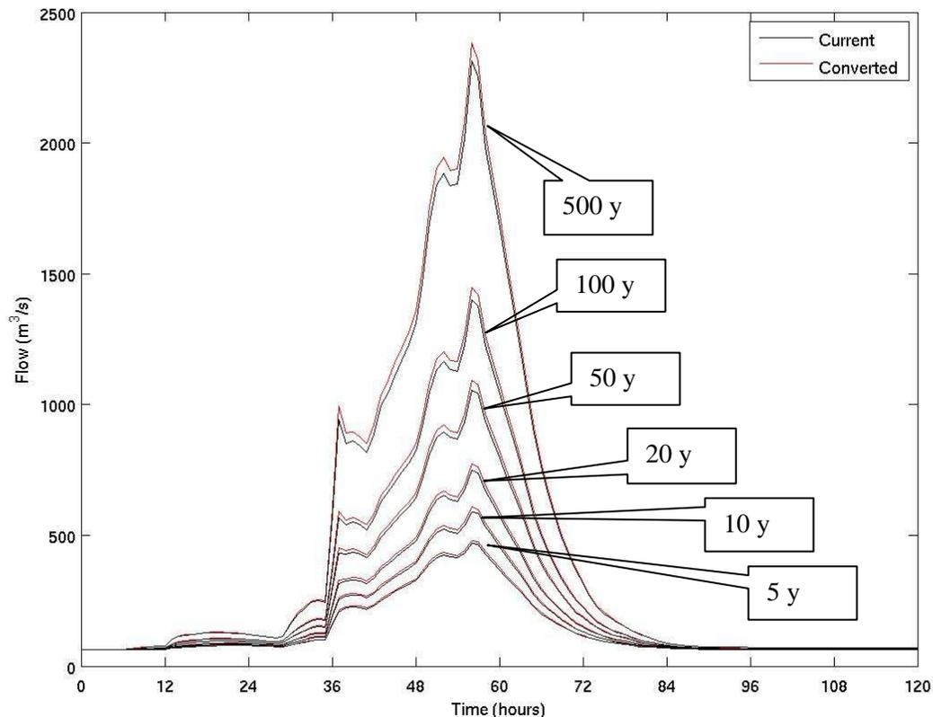
**Figure 30:** Simulated Taupo-Karapiro inflow hydrographs for the 6 synthetic rainfall events under current (black) and converted (red) land use scenarios.
