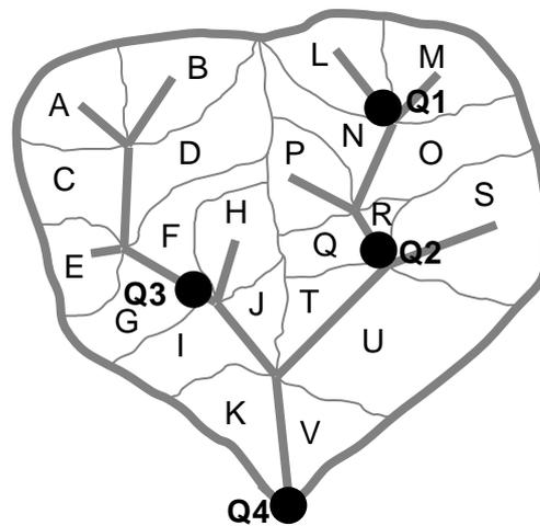
**Figure 1: Schematic of TopNet model: Each letter indicates a sub-catchment, and the symbols Q1 – Q4 indicate the location of flow recording sites.**
