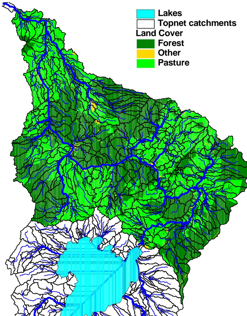
**Figure 3:** TopNet model (order 3) of the middle Waikato, with 2001-02 land cover (source: Environment Waikato) and river network also shown.
