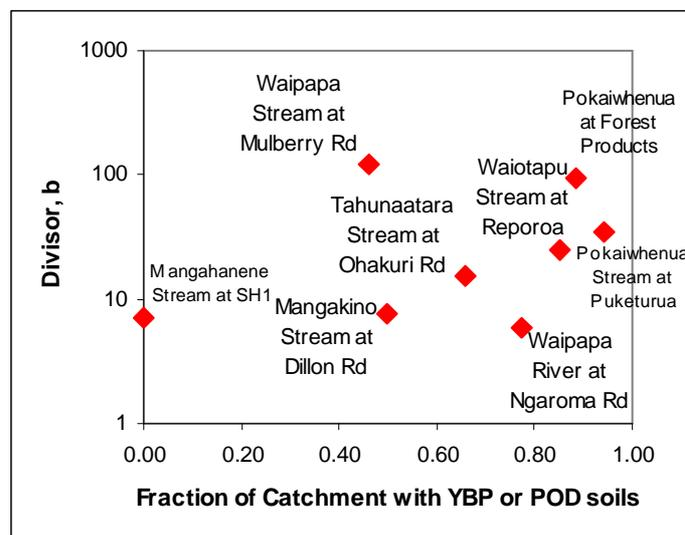
**Figure 8:** Association of Jowett’s divisor *b* (used as a measure of catchment responsiveness) with fraction of catchment containing YBP or POD soils. High values of *b* indicate less responsive catchments. See text for discussion of outlier.
