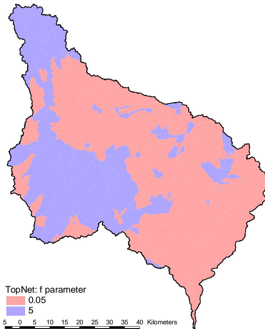
**Figure 10:** Spatial distribution of effective depth (m<sup>-1</sup>) of soil for subsurface flow (TopNet TOPMODF parameter) as applied in the simulation model. The blue areas are predicted by TopNet to be more responsive (for flooding) than the pink areas.
