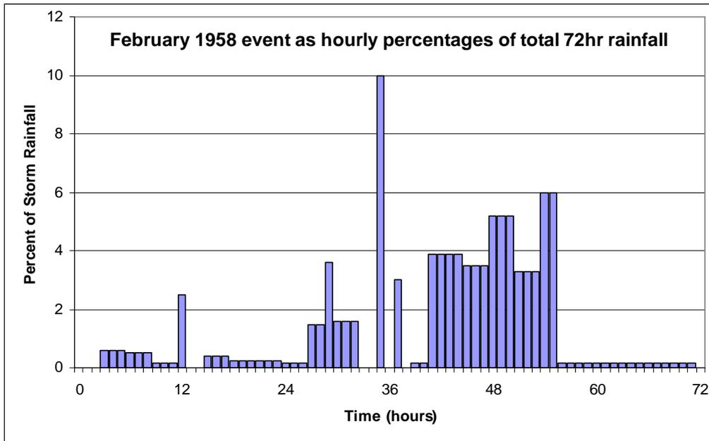
**Figure 20:** Storm rainfall profile for the February 1958 as applied to model land use change impacts.
