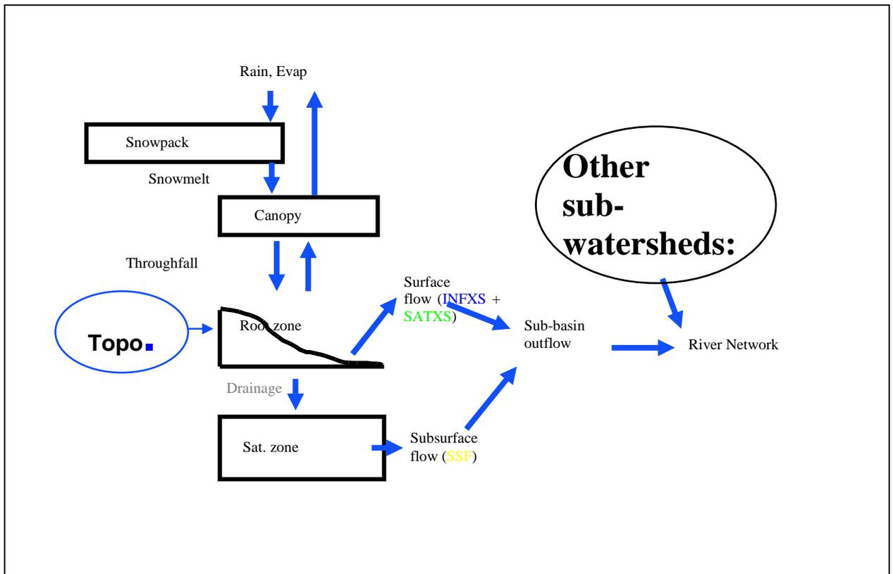
**Figure 2: Overview of TopNet model structure, showing the snowpack, canopy, root zone, saturated zone and river network components of the model. Arrows indicate flows of water from one model component to another. The abbreviations INFXS, SATXS and SSF (and associated colour-coding) are used later in the report.**
