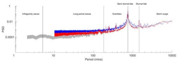
Figure 7. Spectra for Manu Bay tide gauge data for 1-minute resolution data recorded between October 2012 and October 2013 pre-aperture installation (grey line), the 1-minute dataset resampled at 5 minutes (red line) and the 5-minute resolution data recorded between July 2019 and July 2020 post-aperture installation (blue line).
