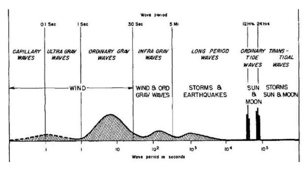
Figure 2. Classification of ocean processes according to wave period and the wave forming factors. The relative wave energy is shown by the curve (Munk, 1950).
