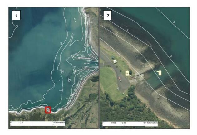
Figure 6. Aerial photo image of Manu Bay tide gauge location showing the wider area (a) and the Manu Bay breakwater (b) with the bubbler (i) and the tide gauge instrumentation (ii). Extent of (b) is shown as a red box (a). Depth contours are in metres below MVD-53 from a compilation of all available bathymetry in the Waikato region (Gardiner and Jones, 2020).
