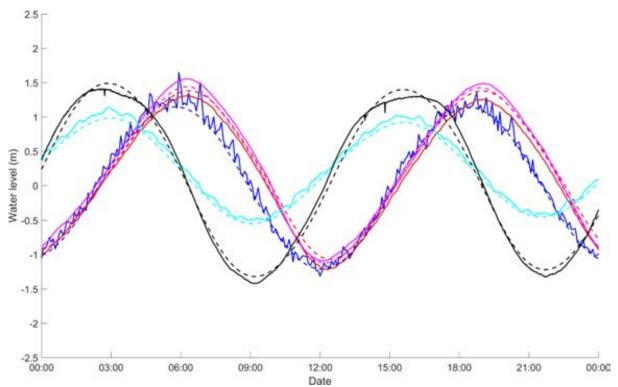
Figure 4. Representative tidal cycle from each gauge. The water level is measured relative to Moturiki Vertical Datum-1953 (MVD-53) at Manu Bay (blue), Raglan Wharf (red), Kawhia Wharf (purple) and Whitianga Wharf (cyan) and TVD-52 at Tararu (black). lines show gauge data (at original sampled frequency) and dashed lines show water level due to tidal processes only (resampled at 10 minutes), see Section 3.1 for details.
