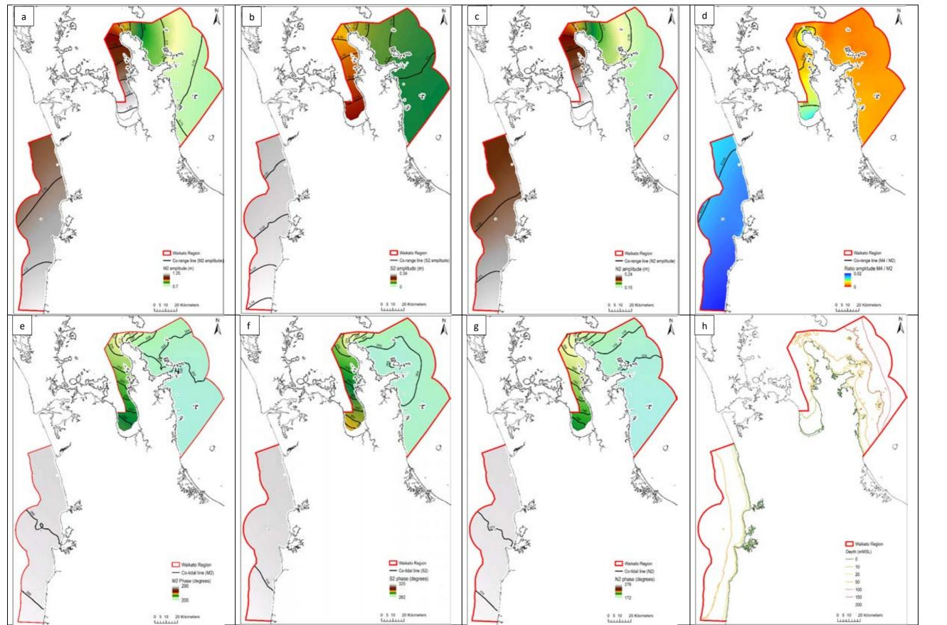
Figure A. 1. Co-range and co-tidal charts showing M2 amplitude (a) and phase (e), S2 amplitude (b) and phase (f), N2 amplitude (c) and phase (g) and M4/M2 amplitude ratio (d) from a regional tidal model (MSL, 2017). Amplitude is the half-range of the constituent (metres) and phase is the timing of the crest of the tide relative to Coordinated Universal Time (degrees). Regional bathymetry (h) from a compilation of all available bathymetry in the Waikato region (Gardiner and Jones, 2020).
