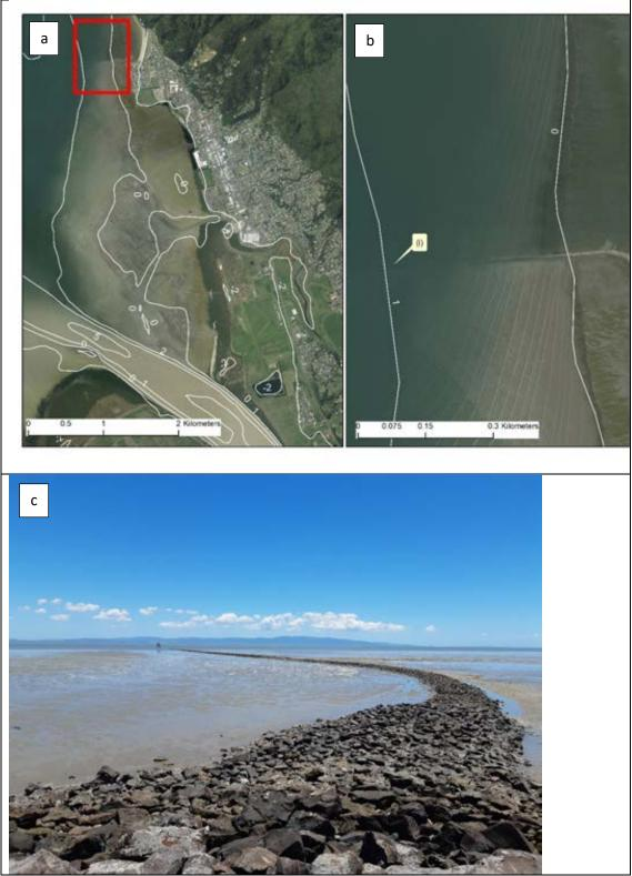
Figure 17. Tararu tide gauge location showing the wider area (a) and platform (b and c) with the tide gauge instrumentation (i). Extent of (b) is shown as a red box (a). Depth contours are in metres below Auckland Vertical Datum 1946 (AVD-46) from a compilation of all available bathymetry in the Waikato region (Gardiner and Jones, 2020). AVD-46 is 0.1278 m below Tararu gauge zero datum (TVD-52) as surveyed on installation. Ongoing subsidence of gauge means that gauge zero is no longer at TVD-52.
