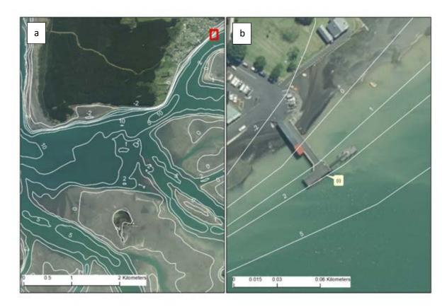
Figure 13. Aerial photo image of Kawhia Wharf tide gauge location showing the wider area (a) and Kawhia Wharf (b) with the bubbler location (i). Extent of (b) is shown as a red box (a). Depth contours are in metres below to MVD-53 from a compilation of all available bathymetry in the Waikato region (Gardiner and Jones, 2020).
