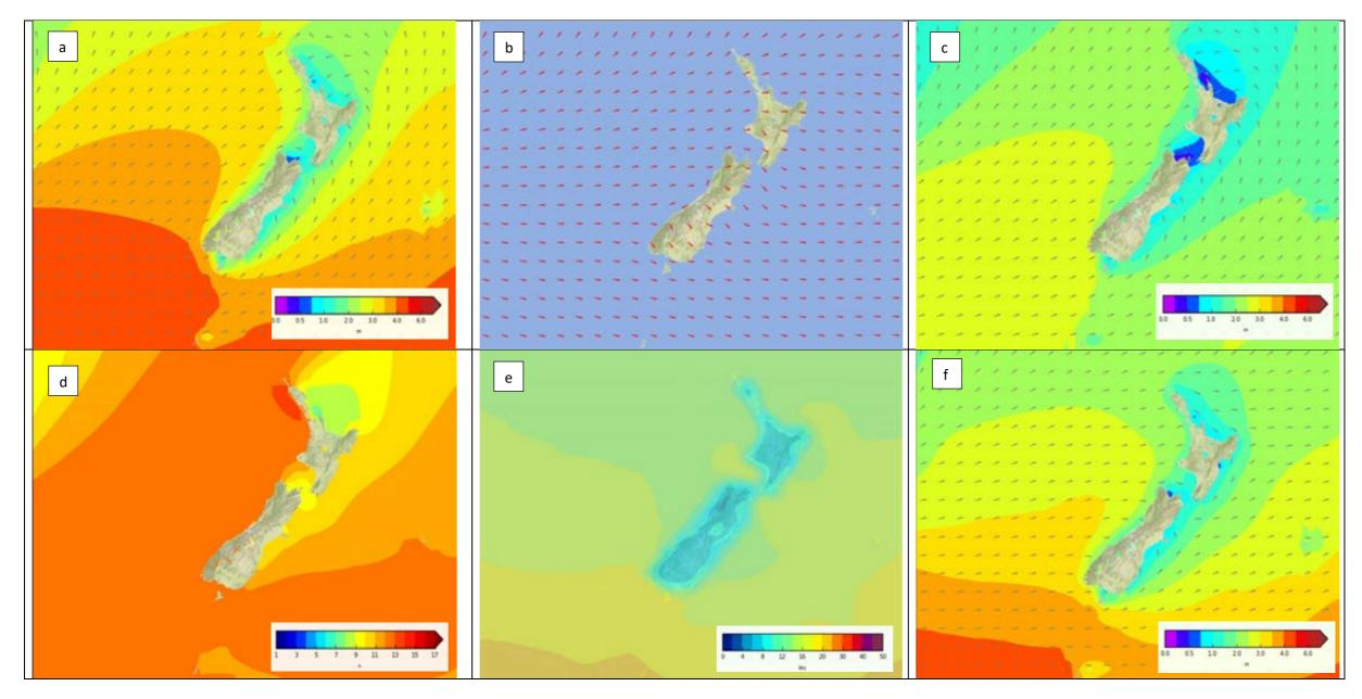
Figure A. 2. Modelled hindcast data showing Mean significant wave height and direction (a), Mean wind direction (b), Mean swell wave height and direction (c), Mean peak period (d), Mean wind speed (e), Mean sea wave height and direction (f). Data from MetOcean View (https://metoceanview.com).
