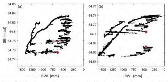
**Figure 5** Half-hourly values of peat surface elevation (SE) plotted against relative water level (RWL) at (a) Site SD hump and (b) Site BD hump, for the measurement period (1 March 2019 - 1 August 2020). Red diamonds indicate the same RWL in July 2019 and July 2020, but different SE representing current best estimate of the irreversible subsidence rate. Note that the values on the Y axes differ between sites, but the ranges are the same.
