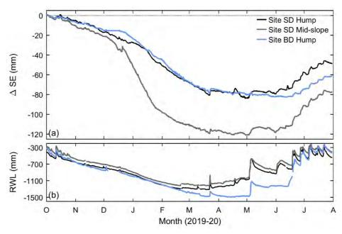
**Figure 4** Six-hourly mean changes in (a) total peat surface elevation ( $\Delta$  SE) based on data from the paired pressure transducers at Sites SD (hump and mid-slope) and BD (hump), and (b) relative water level (RWL) during the period 1 October 2019 and 1 August 2020.
