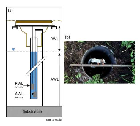
Figure 1 (a) Cross-sectional diagram of the paired pressure transducer method, showing the steel rod bridging the aluminium channels either side of the dipwell, from which the RWL probe is suspended, and the vertical benchmark rod from which the AWL probe hangs, (b) vertical photograph of a dipwell containing paired pressure transducers.
