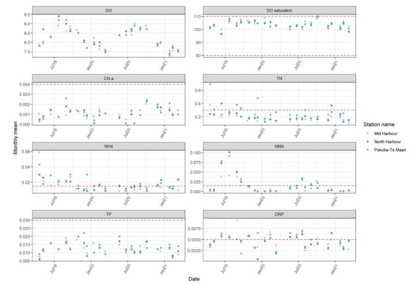
Figure C-11-10. Chemical water quality parameters over time for Aotea Harbour. Dashed red lines denote ANZECC (2000) guidelines values. For parameter units refer to table 2-1.
