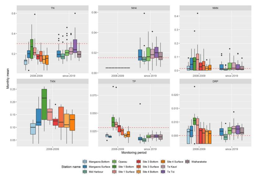
Figure 6-9. Distribution of chemical estuarine water quality monitoring data per monitoring period for Kawhia Harbour Part 2. See figure 2-2 for boxplot range definition. Dashed red lines represent ANZECC guideline limits for the applicable parameter (see Table 2-2). For parameter units refer to table 2-1.
