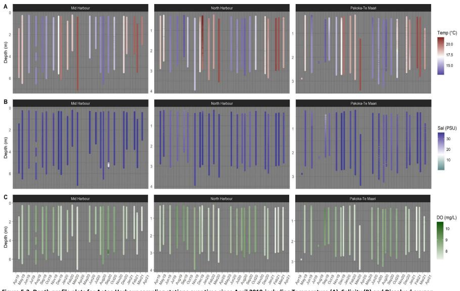
Figure 5-3. Depth profile plots for Aotea Harbour sampling stations over time since April 2019 including Temperature (A), Salinity (B) and Dissolved oxygen concentration (C).
