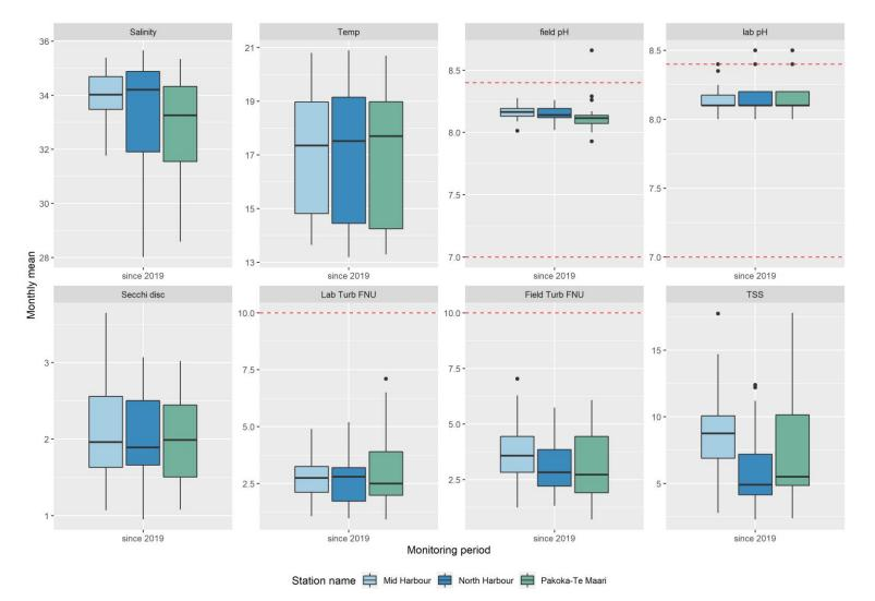
Figure 5-4.Distribution of physical estuarine water quality monitoring data per monitoring period for Aotea Harbour. See figure 3-2 for boxplot range definition. Dashed red lines represent ANZECC guideline limits for the respective parameter (Table 3-2). For parameter units refer to table 2-1.
