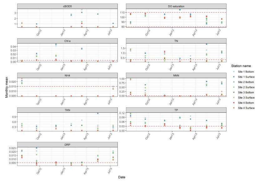
Figure C-11-2. Chemical water quality parameters over time for Port Waikato. Dashed red lines denote ANZECC (2000) guidelines values. For parameter units refer to table 2-1.
