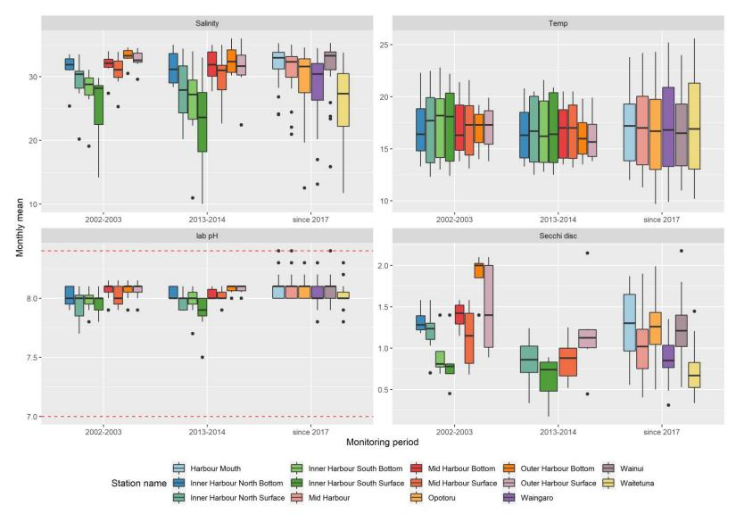
Figure 4-6. Distribution of physical estuarine water quality monitoring data per monitoring period for Whāingaroa Harbour Part 1. See figure 3-2 for boxplot range definition. Dashed red lines represent ANZECC guideline limits for the respective parameter (Table 3-2). For parameter units refer to table 2-1.
