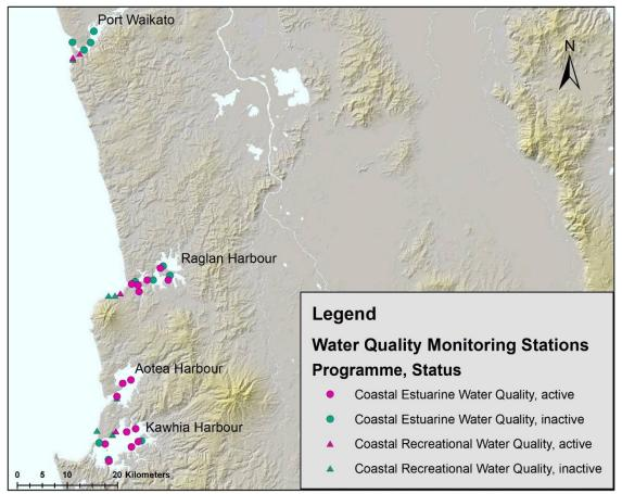
Figure 1-1. Water quality monitoring stations for the West Coast of the Waikato Region for coastal estuarine water quality (ecological health) and coastal recreational water quality. Active stations are currently monitored, and current data is available. Only historical data is available for inactive stations.
