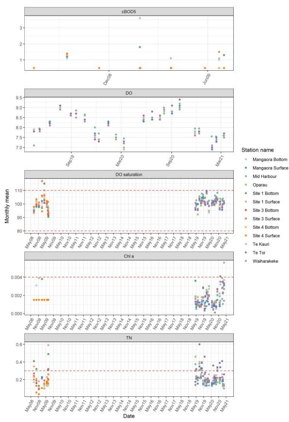
Figure C-11-14. Chemical water quality parameters over time for Kawhia Harbour Part 1. Dashed red lines denote ANZECC (2000) guidelines values. For parameter units refer to table 2-1.
