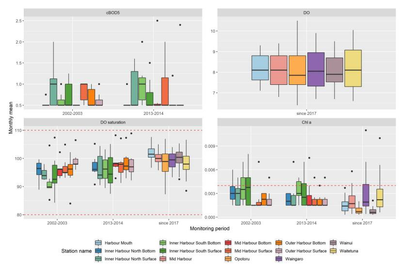
Figure 4-8. Distribution of chemical estuarine water quality monitoring data per monitoring period for Whāingaroa Harbour part 1. See figure 3-2 for boxplot range definition. Dashed red lines represent ANZECC guideline limits for the respective parameter (Table 3-2). For parameter units refer to table 2-1.
