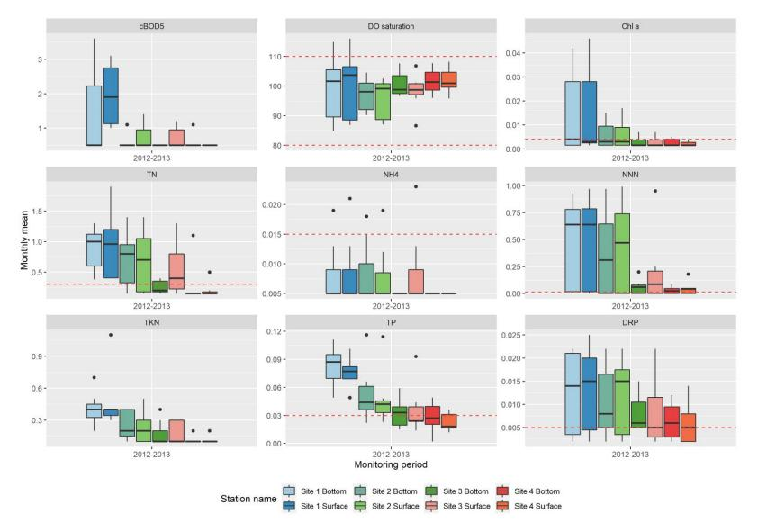
Figure 3-3. Distribution of chemical estuarine water quality monitoring data per monitoring period for Port Waikato. See figure 3-2 for boxplot range definition. Dashed red lines represent ANZECC guideline limits for the applicable parameter (see Table 2-2). For parameter units refer to table 2-1.
