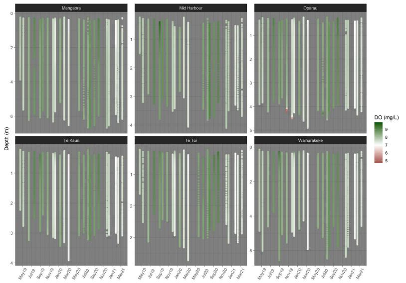
Figure 6-5. Dissolved oxygen-depth profile plots for Kawhia Harbour sampling stations over time since April 2019.
