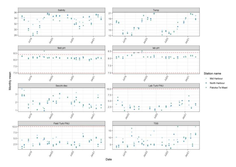
Figure C-11-9. Physical water quality parameters over time for Aotea Harbour. Dashed red lines denote ANZECC (2000) guidelines values. For parameter units refer to table 2-1.
