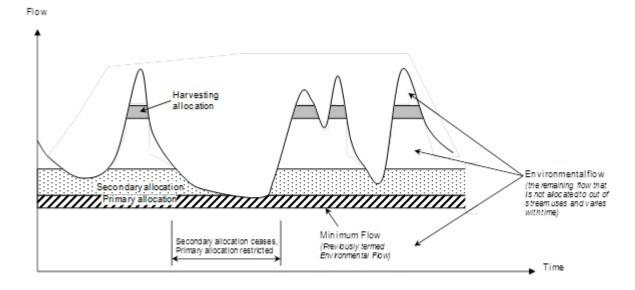
Figure 35: Diagram of hydrograph and were minimum flows, primary and secondary flows and water harvesting flows fit within it.
