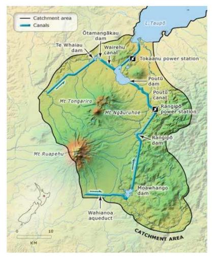
Figure 15: Extent of Tongariro Power Scheme and location of key infrastructure elements. Source: www.teara.govt.nz/en/map/21656/tongariro-power-scheme
