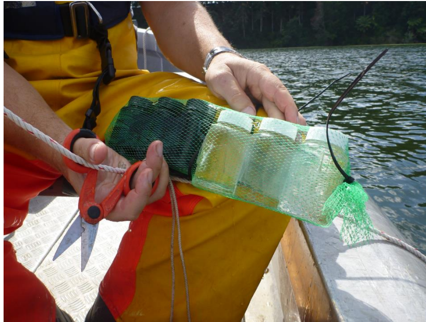
Figure 4: PPR bottles assembled in a net bag attached to an incubation line ready for deployment. The dark control bottles were painted black and covered with black tape.
