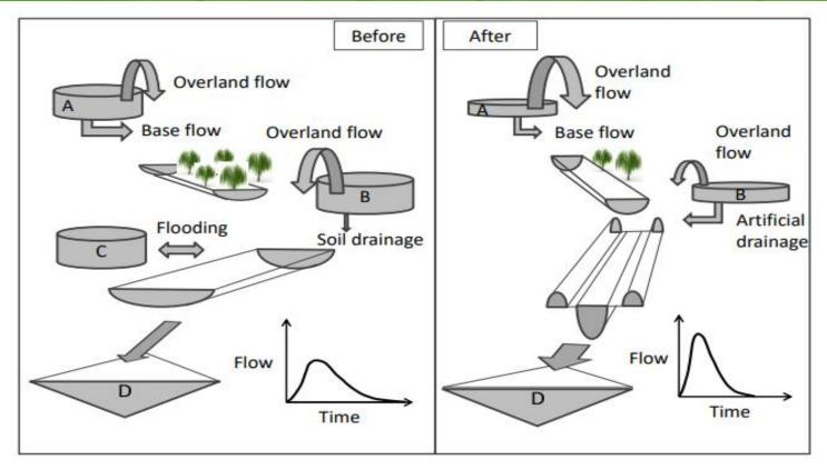
Conceptual alterations to the hydrology of altered catchments. A and B represent catchment water storage capacity in hill country; C represents flood plain storage and D represents estuary or harbour.
