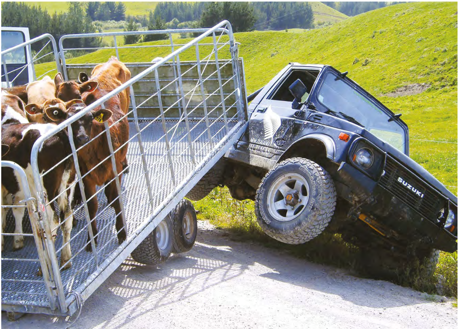
The towing vehicle must match the load – here the coupling has sheared
