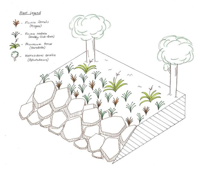
Sample layout of the type of planting that could be done along the crest of the new seawall, and where possible, extending down the face of the wall. This incorporates the existing Pōhutukawa trees present along some parts of the wall and introduces native dune species to encourage an increase in biodiversity in this area. Native plants will further attract native bird and insect species.
