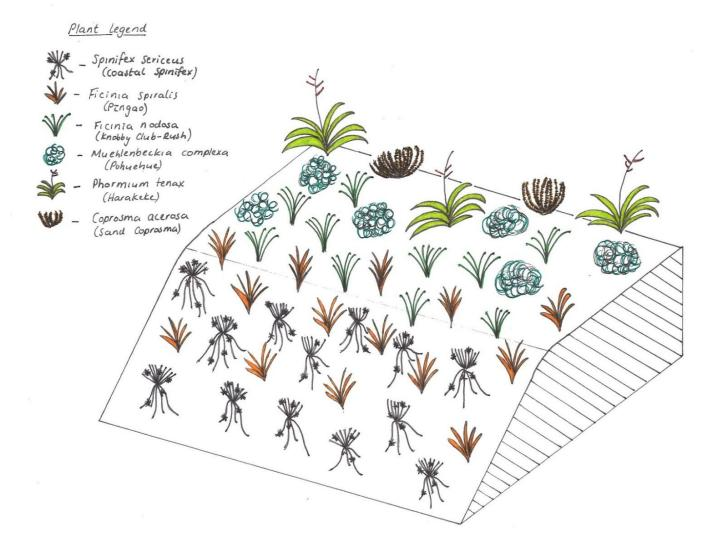
Sample layout of the type of planting that could be done on the natural dune system at the southern end of the seawall. Plants utilised on the face of the foredune are those with strong sand binding qualities that are more resistant to sand movement. These species will help stabilise the foredune. All these species are well adapted to the changing conditions of coastal environments.
